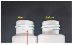
Second printing position pin provides better support during the production. 牙口位置的第二道定位校正設計提高印刷時的定位準確度
